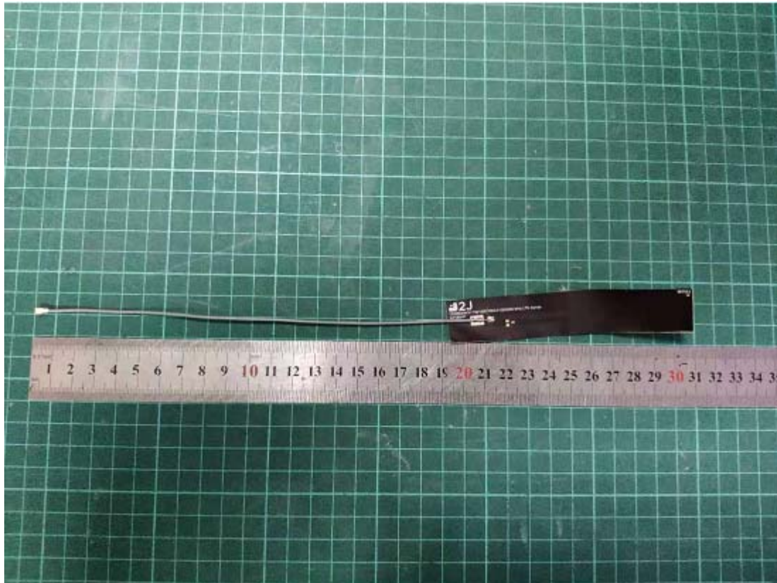
Typical external antenna
