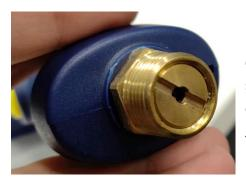
Here is the description of the air pressure connection as you may want to connect another air pressure hose and not the one delivered by default. However, it is mandatory to make sure the air hose and pressure stick are certified in your country of usage and given for a maximum of 20bar or more.
