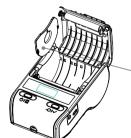
Insert the paper roll with the printing side of the first label face down. Position the baffle to hold the roll against the right side of the printer.
