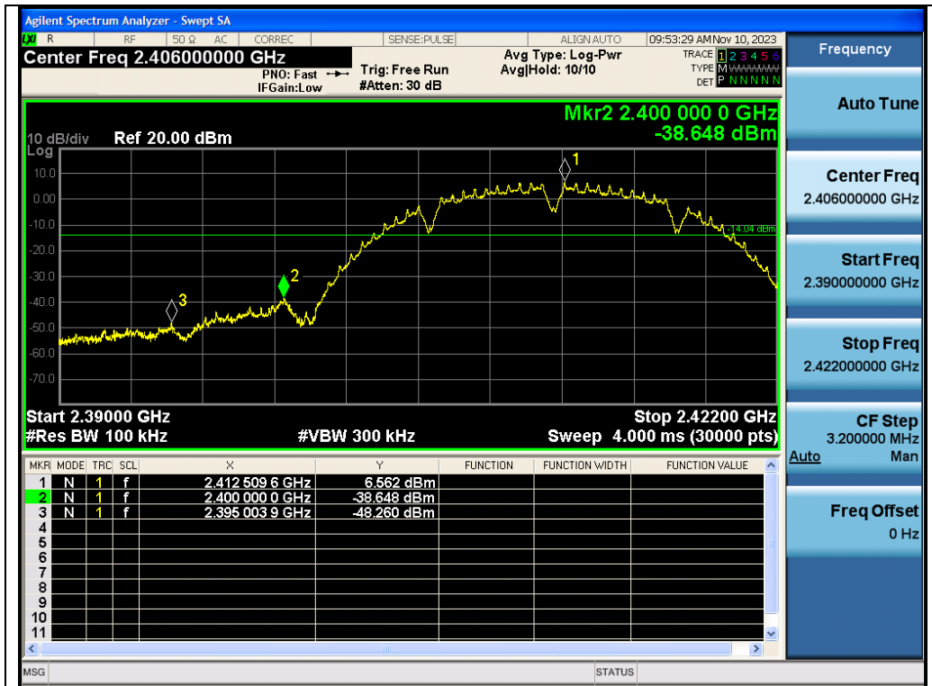
Test_Graph_802.11b_ANT1_2412_1Mbps_Lower Band Edge Emissions
