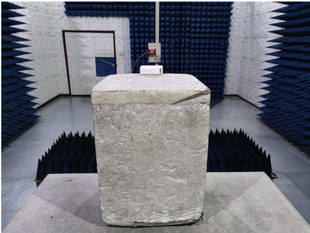
RADIATED EMISSION TEST SETUP ABOVE 1GHz
