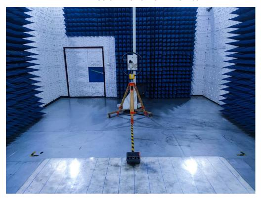
RADIATED EMISSION TEST SETUP BELOW 1GHz
