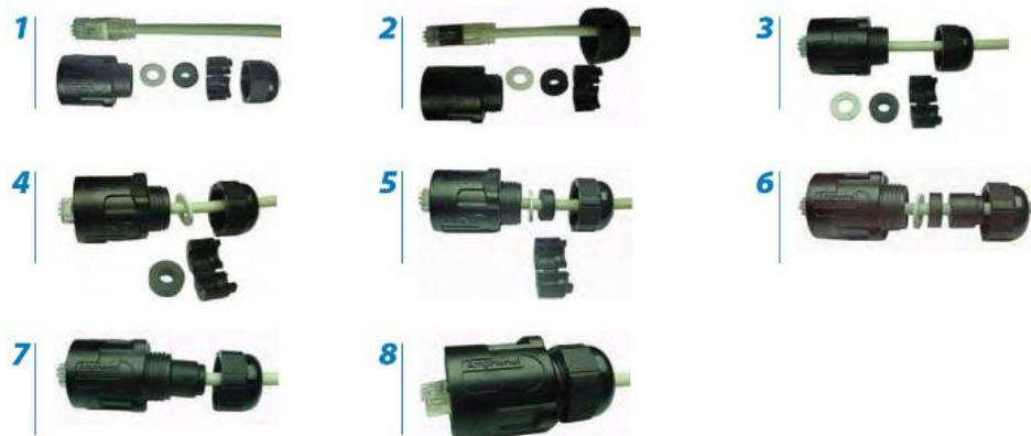
Figure 3: Steps to dress the Ethernet cable with the Amphenol connector housing
