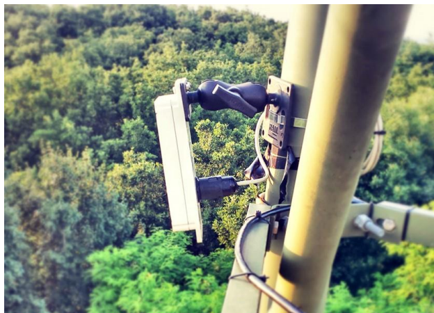
Figure 4 – View of the GATEWAY attached on a pole with RAM mount joints
