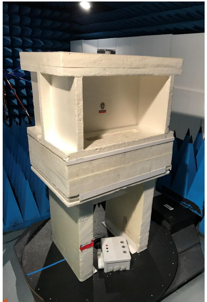
Test setup in anechoic chamber (test setup > 1GHz)
