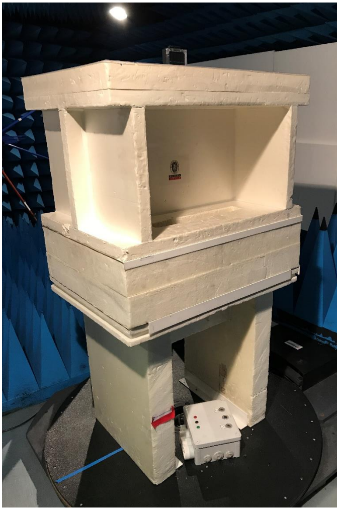
Test setup in anechoic chamber (test setup > 1GHz)
