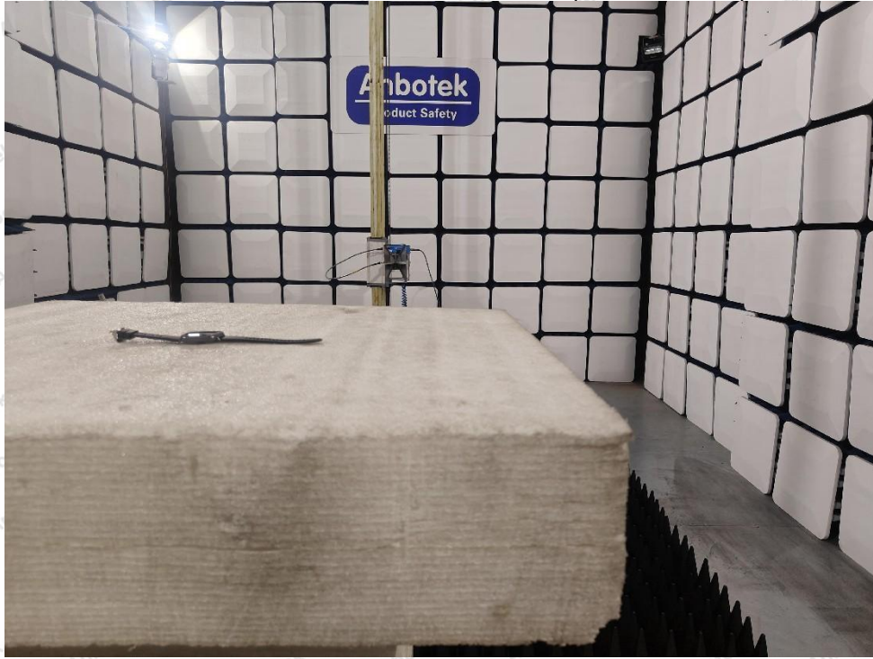
Photo of Radiation Emission Test (above 1GHz)
