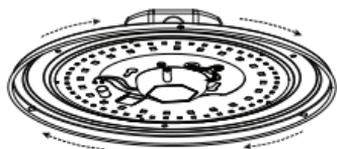
6. Tighten the screws with a screwdriver.
