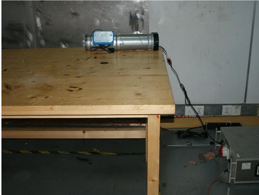
Photograph 1: Set-up for Conducted Emission on AC Mains
