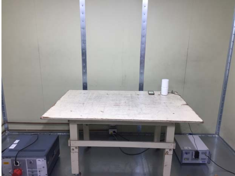
Photograph 3 : Setup for Conducted Emissions
