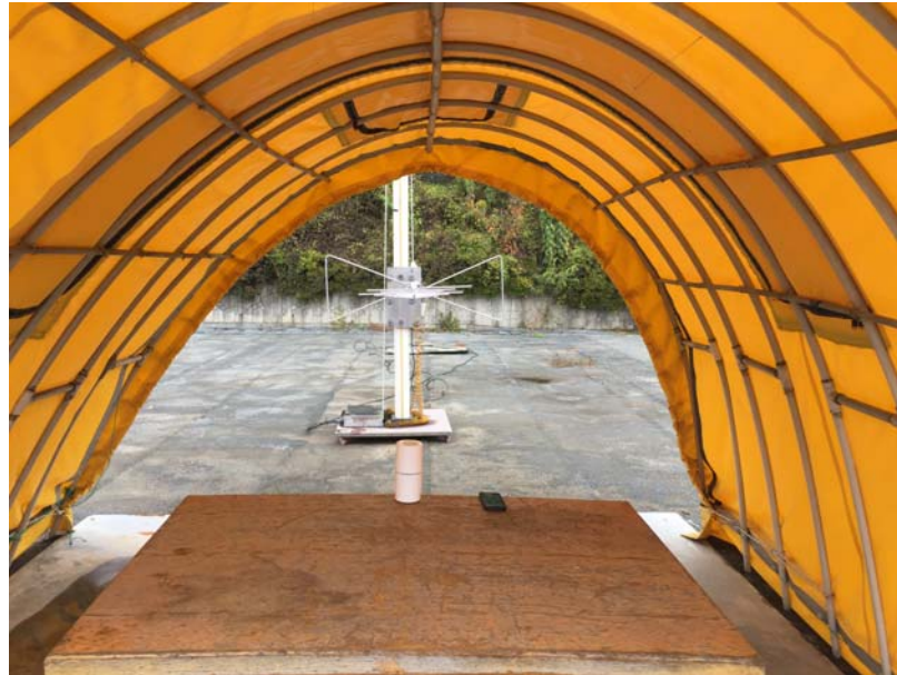
Photograph 2 : Setup for radiated Emissions (above 1 GHz)
