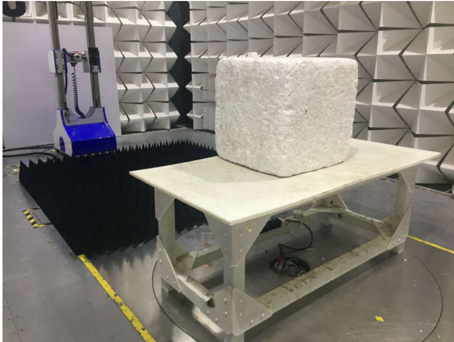
Radiated spurious emission Test Setup-3(Above 1GHz)
