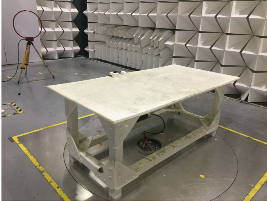
Radiated spurious emission Test Setup-1(Below 30MHz)
