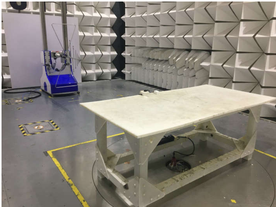
Radiated spurious emission Test Setup-2(Below 1GHz)
