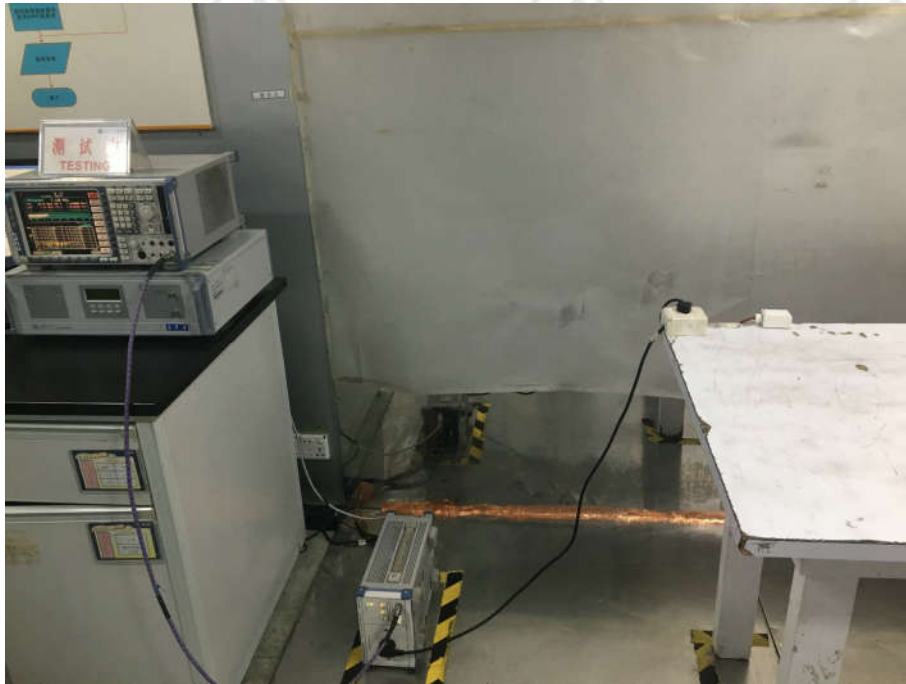
Conducted Emissions Test Setup
