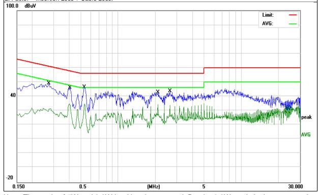
Note: The mode of 5W and 9.9W load has been tested. But the 9.9W mode is the worst mode, just reported the worst data.
