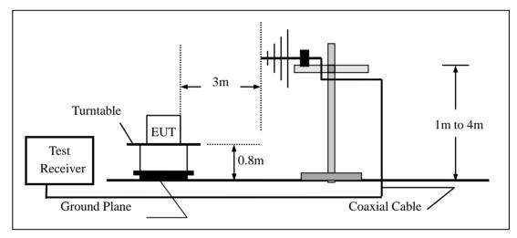
(c) For radiated emissions above 1000MHz
