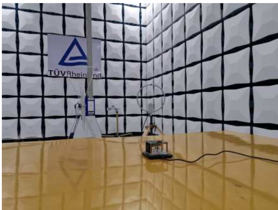
Photograph 1: Set-up photo for Radiated Emission, 9KHz - 30MHz
