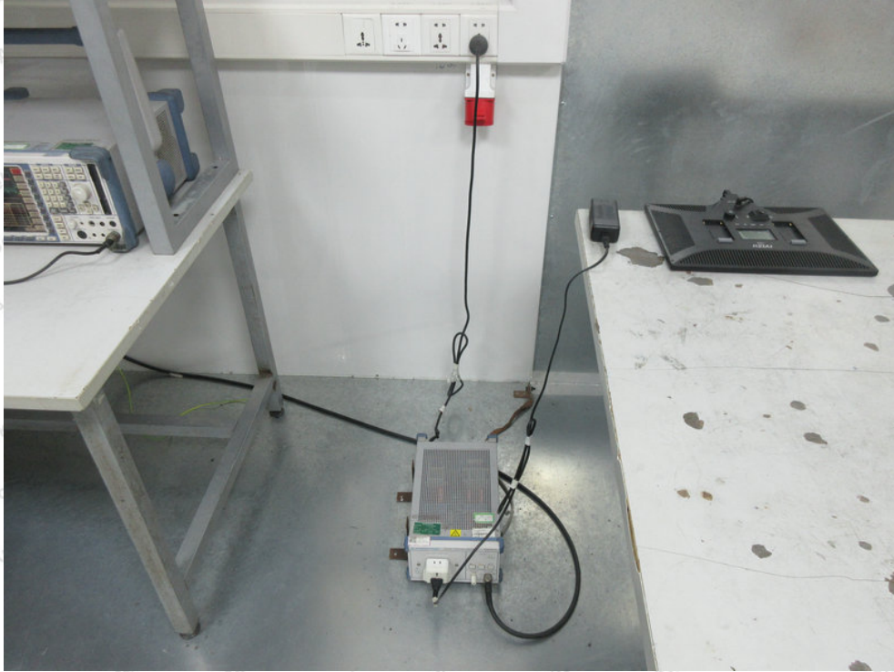
Photo of Power Line Conducted Emission Test
