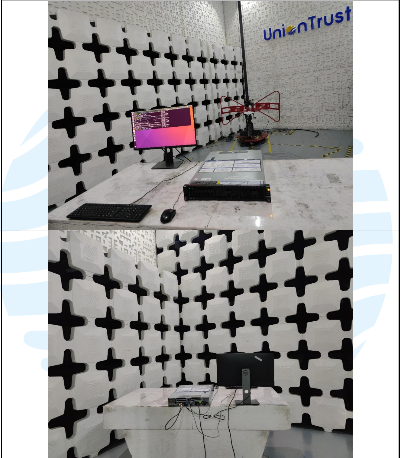
Radiated emission Test Setup-1 (30 MHz~1 GHz)
