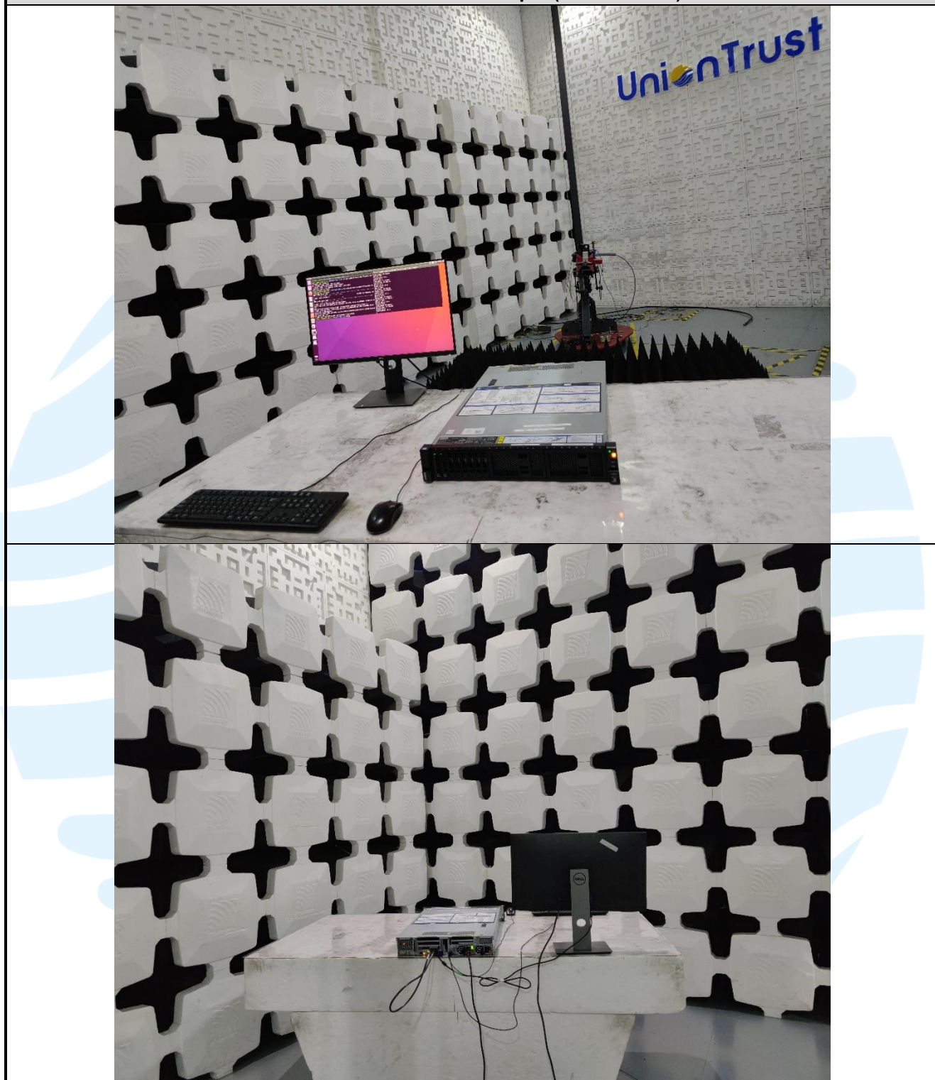
Radiated emission Test Setup-2 (Above 1 GHz)
