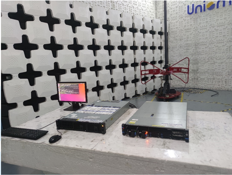
Radiated emission Test Setup (30 MHz~1 GHz)
