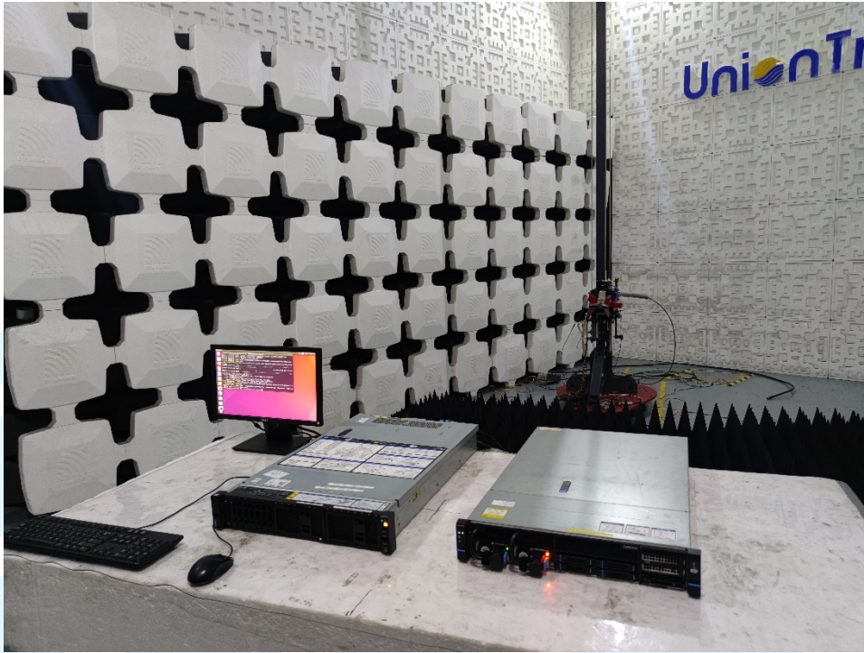
Radiated emission Test Setup (Above 1 GHz)
