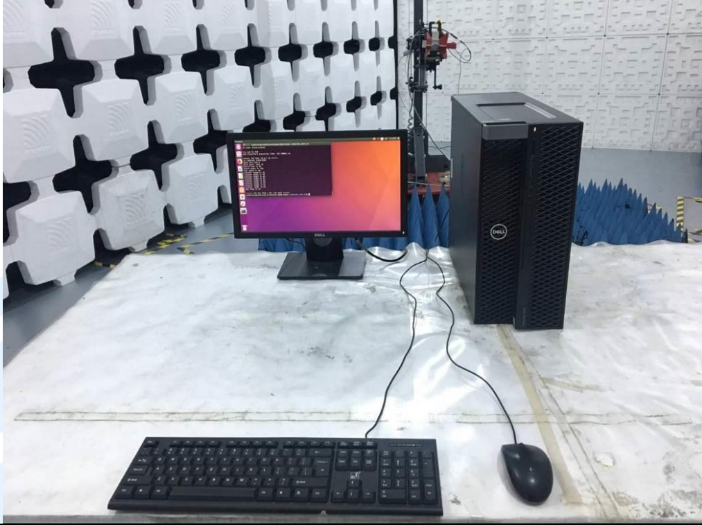
Radiated emission Test Setup-2 (Above 1 GHz)
