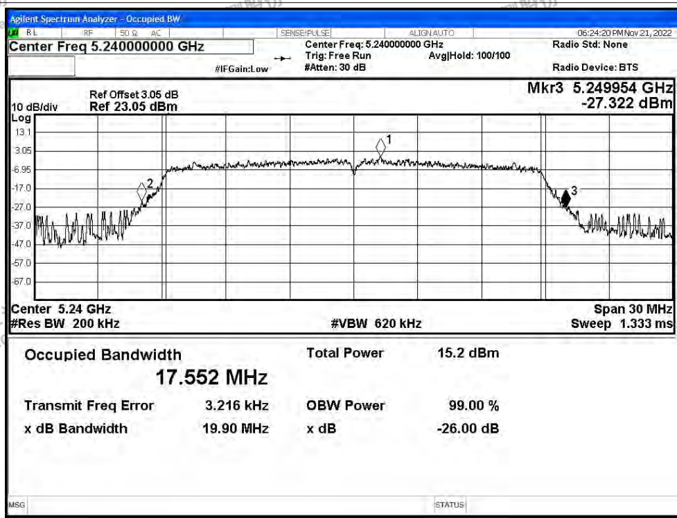
-26dB Bandwidth NVNT n20 5240MHz Ant0
