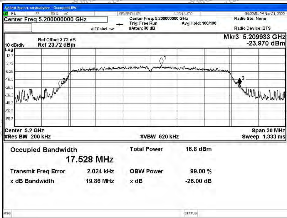
-26dB Bandwidth NVNT n20 5240MHz Ant0
