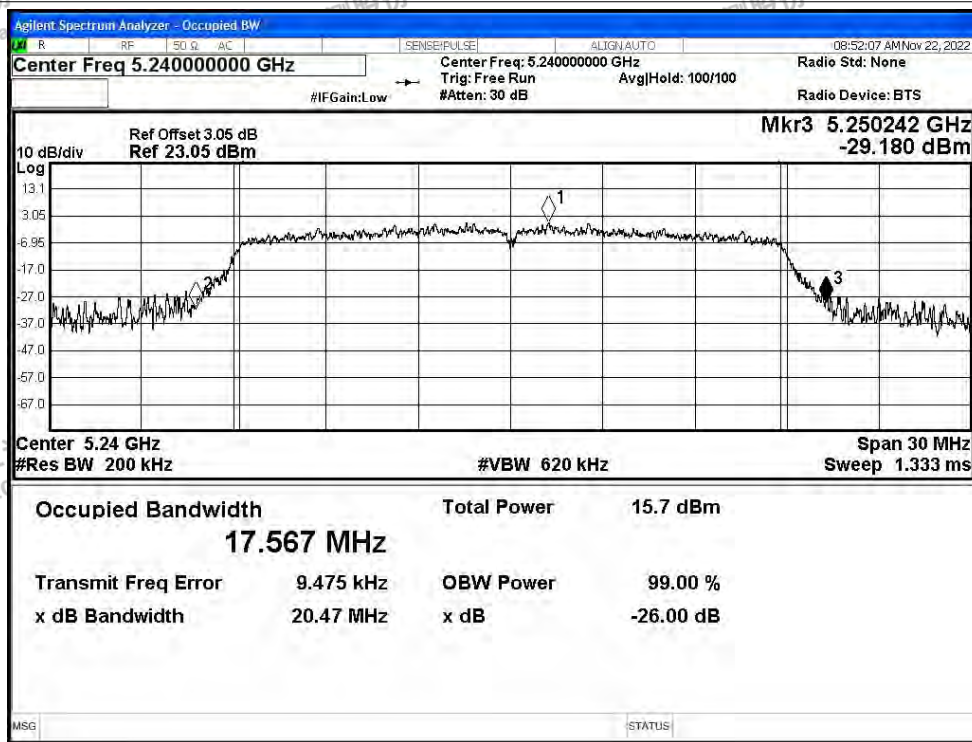
-26dB Bandwidth NVNT n20 5240MHz Ant1
