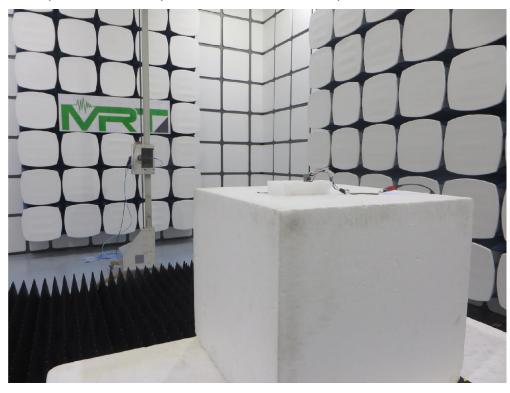
Description: Radiated Spurious Emission Test Setup for  $18\text{GHz} \sim 40\text{GHz}$
