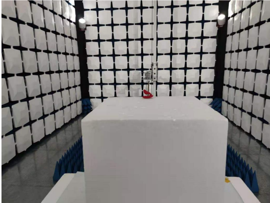
Model: SMV28 Above 1GHz for radiated emission test setup
