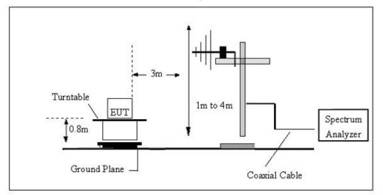
(C) Radiated Emission Test-Up Frequency Above 1GHz
