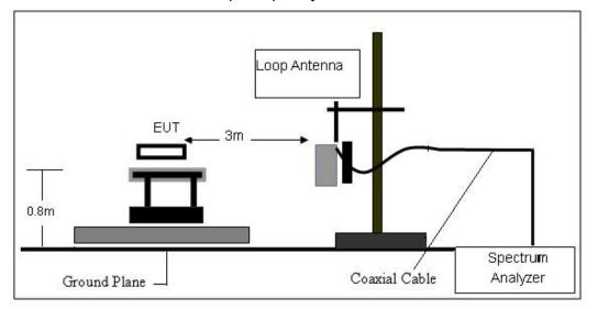
(B) Radiated Emission Test-Up Frequency 30MHz~1GHz
