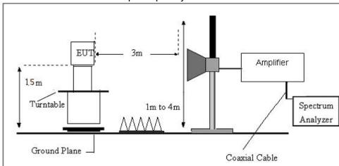
Radiated Emission Test-Up Frequency Above 1GHz
