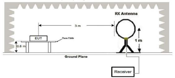
(2) Radiated Emission Test-Up Frequency 30MHz~1GHz
