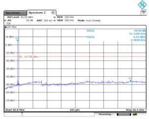
Note: It is not recorded on the report that the reading of emissions are attenuated more than 20 dB below the permissible limits
