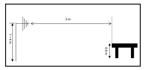
Radiated emission setup, above 1 GHz
