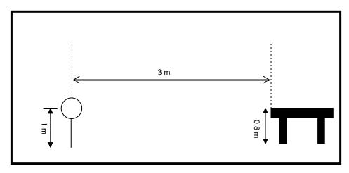
Radiated emission setup, below 1 000 MHz
