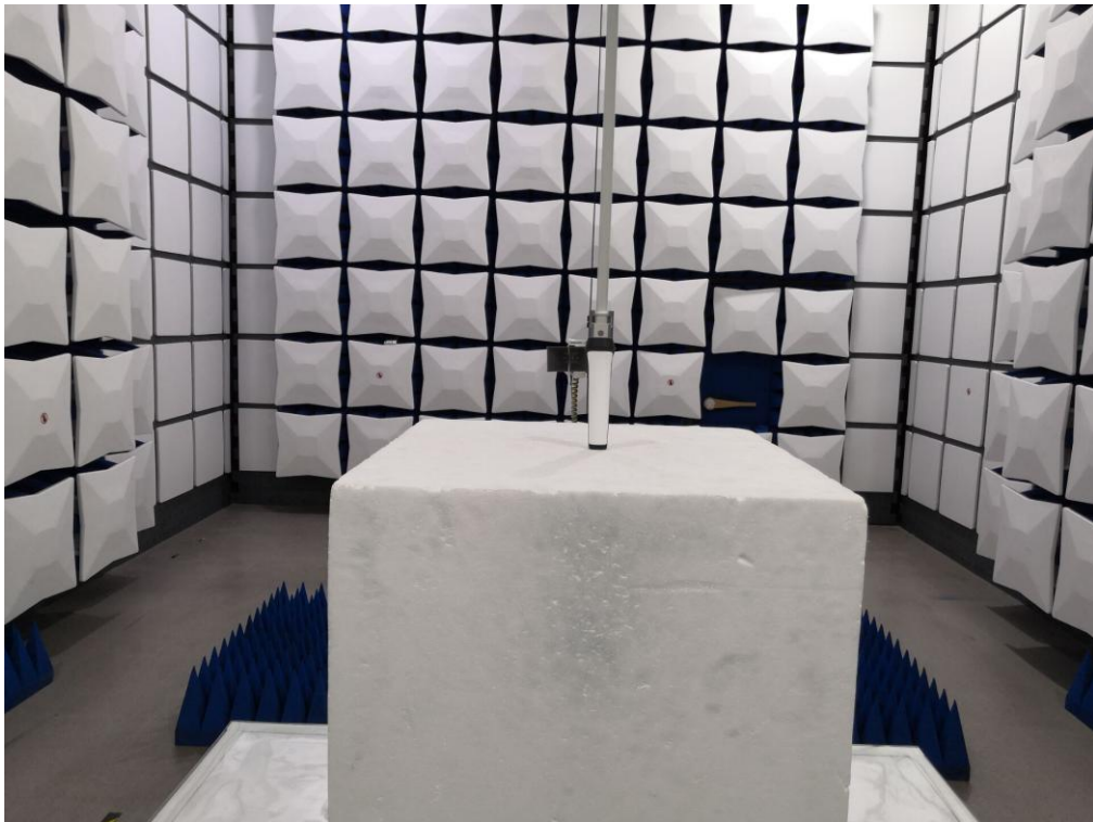
FCC RADIATED EMISSION TEST SETUP ABOVE 1GHZ
