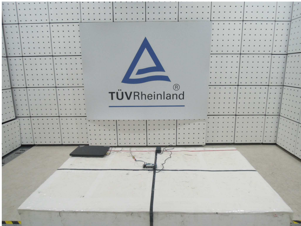
Photograph 1: Set-up for Spurious Emissions (Front View)
