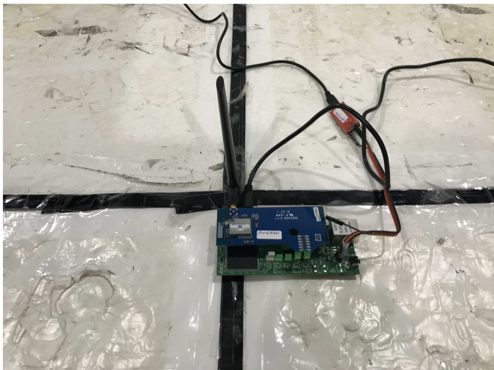
Photograph 4: Set-up for Spurious Emissions (Zoom In)
