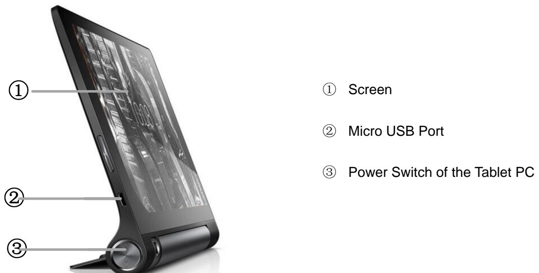
Fig. 3.1 Structure of Tablet PC
