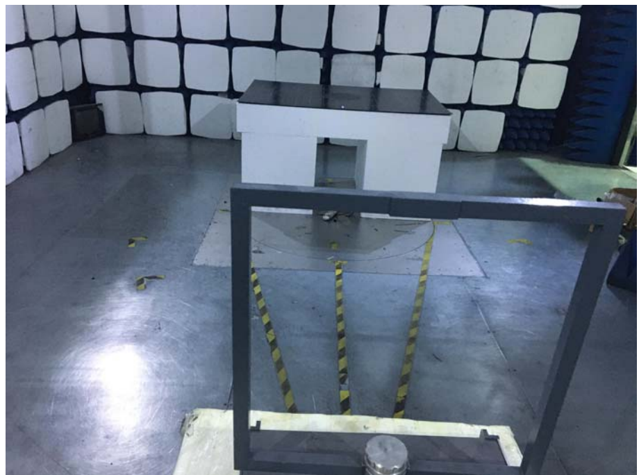
Radiation Emission Test Setup (Below 30MHz)
