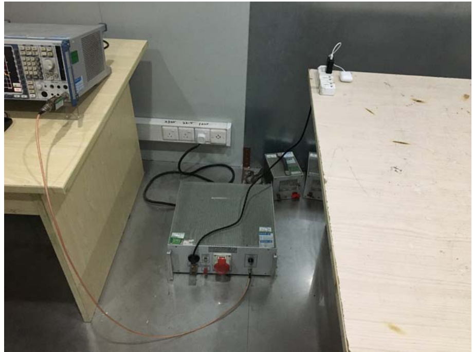
Conducted Emission Test Setup
