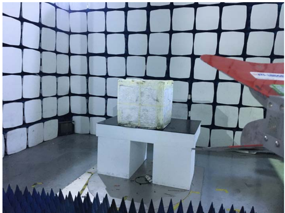
Radiation Emission Test Setup (1GHz to 18GHz)
