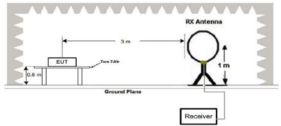
(2) Radiated Emission Test-Up Frequency 30MHz~1GHz
