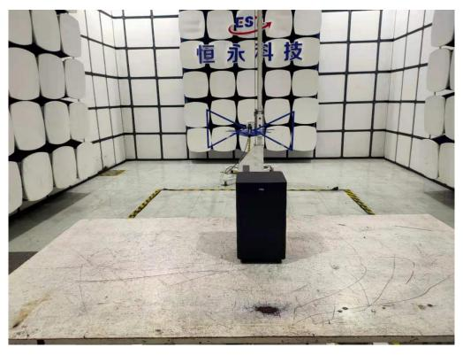
**Radiated Test (Above 1GHz)** M/N:TS8132-SW
