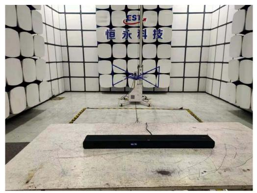
Radiated Test (Above 1GHz) M/N:TS8132
