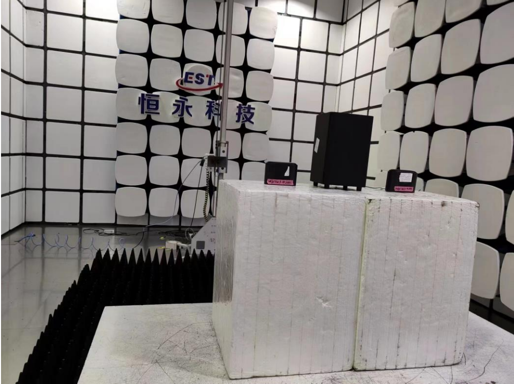
Radiated Test (Above 1GHz)
