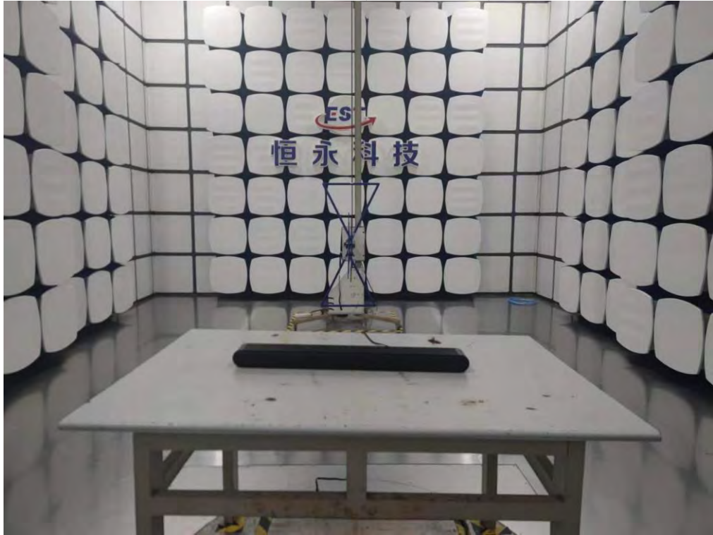
Radiated Test (Below 1GHz)
