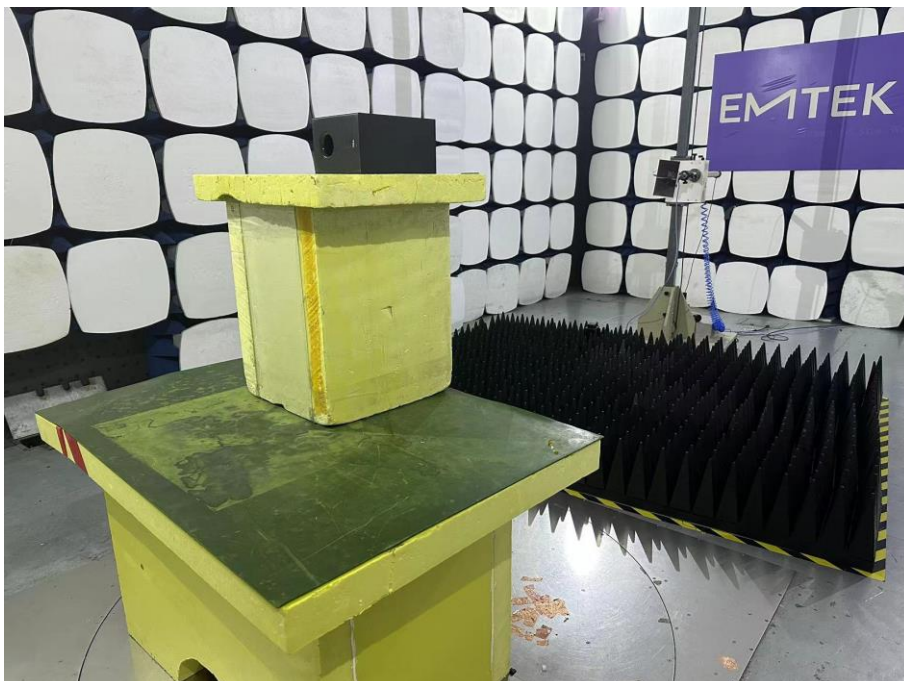
Spurious Emission Test Setup (Above 1GHz)
