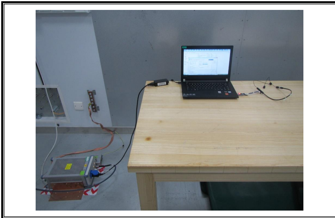
POWERLINE CONDUCTED EMISSIONS MEASUREMENT SETUP
