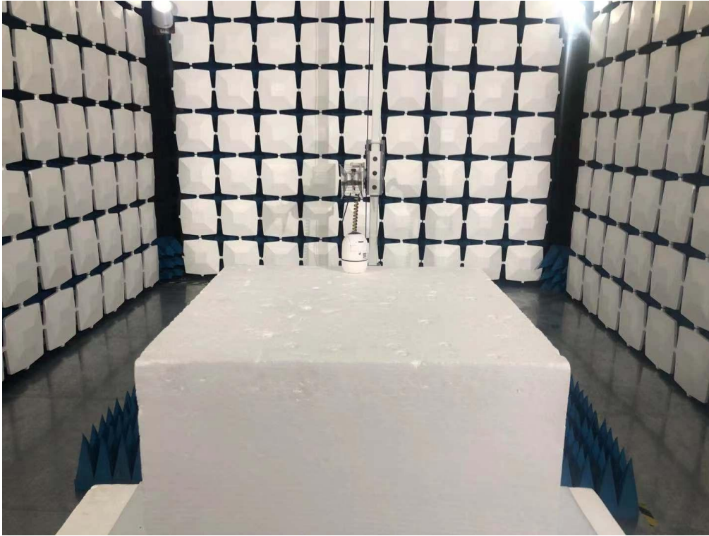
Above 1GHz for radiated emission test setup
