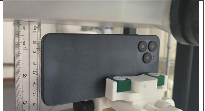
Bottom Side (Separation distance of 10mm)
