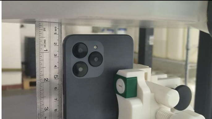
Top Side (Separation distance of 10mm)
