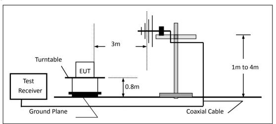
(c) For radiated emissions above 1000MHz
