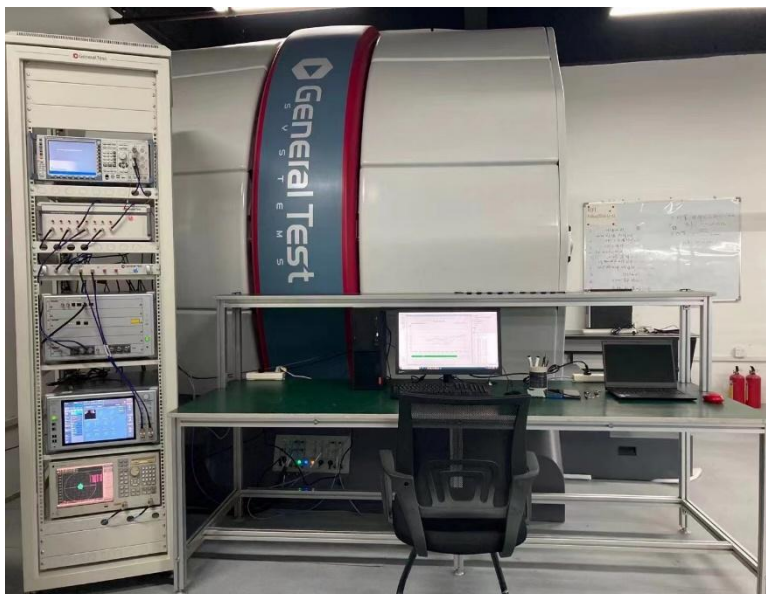
DUT setup photo of free space OTA testing
