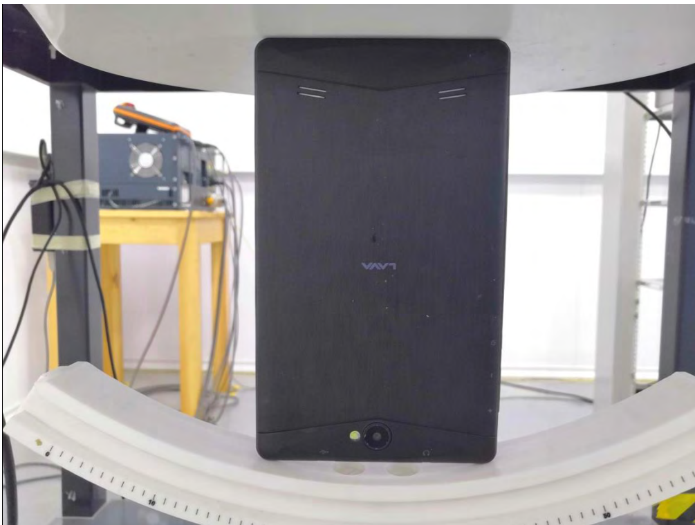
0mm body-worn Bottom Side Setup Photo (hotspot)
