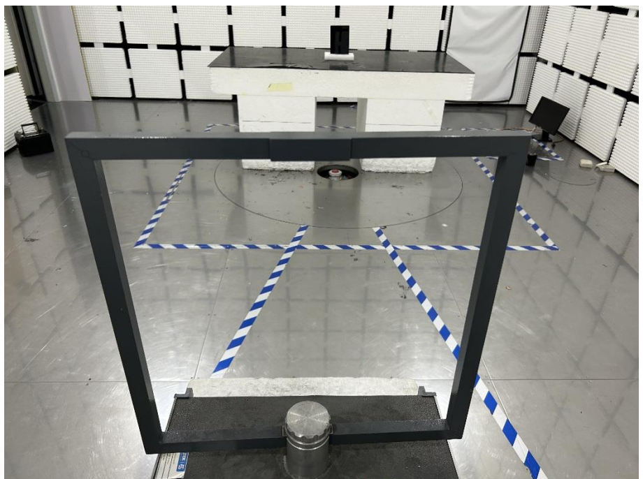
Radiation Emission Test Setup (Below 30MHz)
