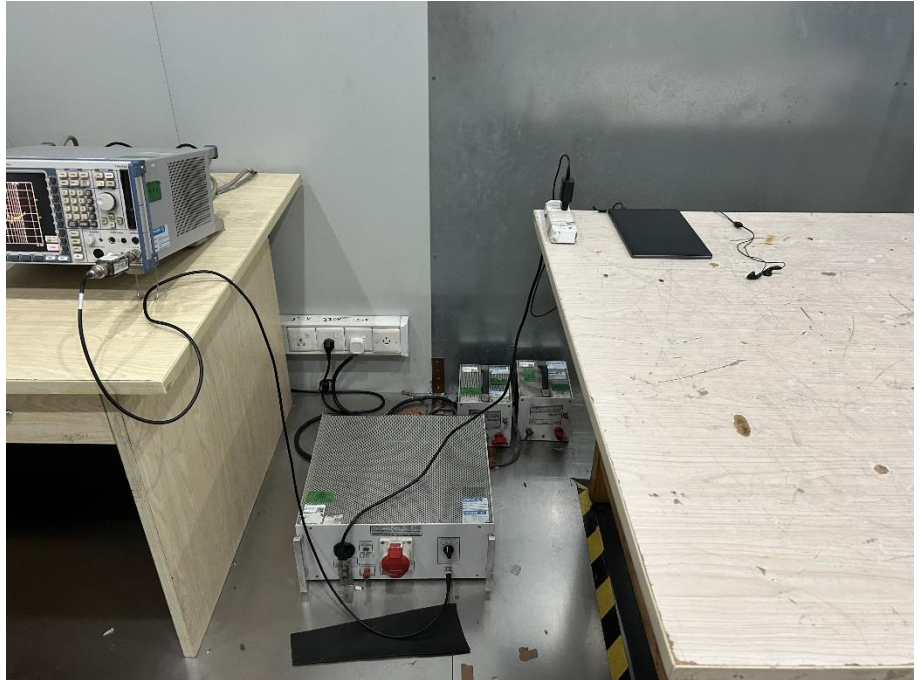
Conducted Emission Test Setup
