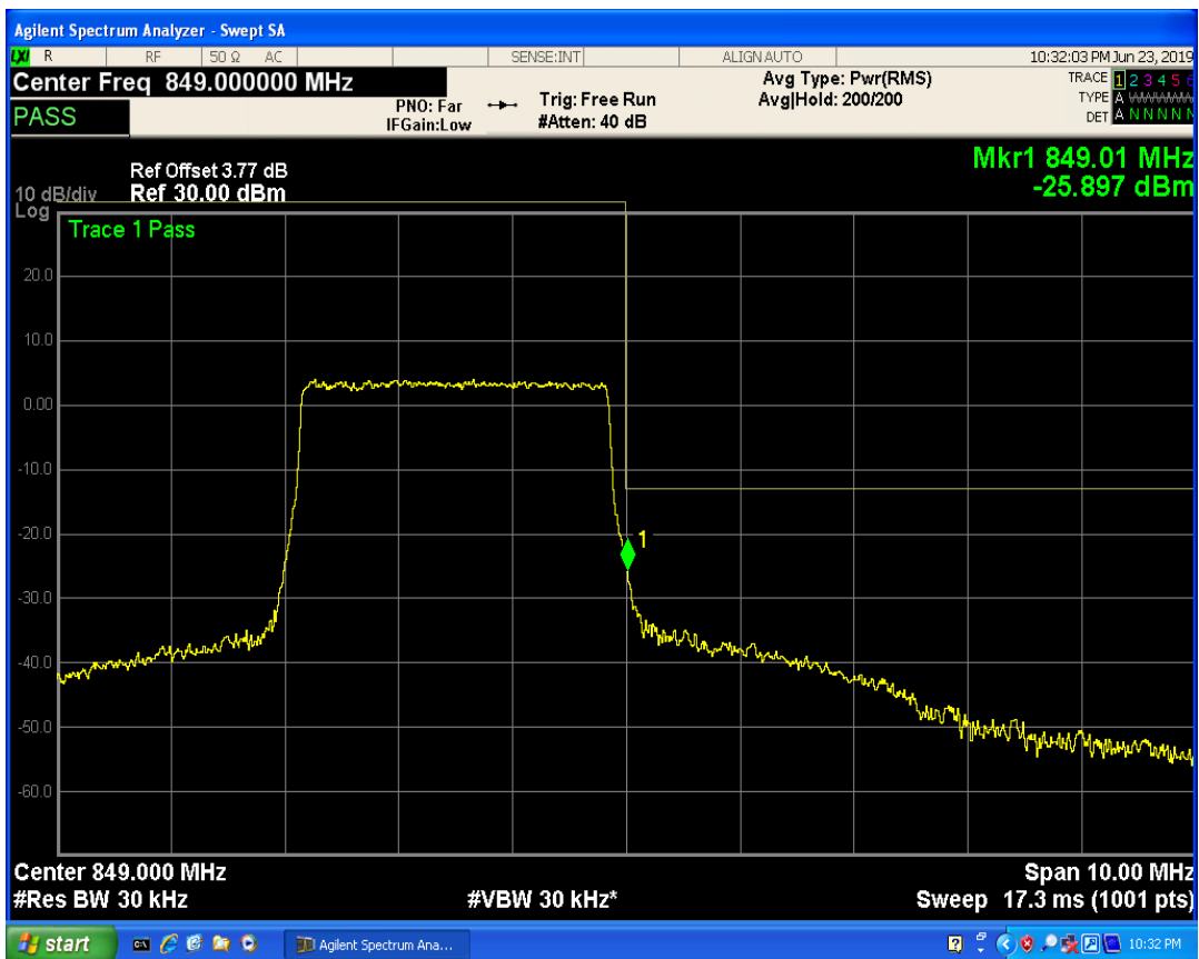
LTE Band5 QAM16 BW=3MHz Channel=20635 RB Size=1 Position=#Mid
