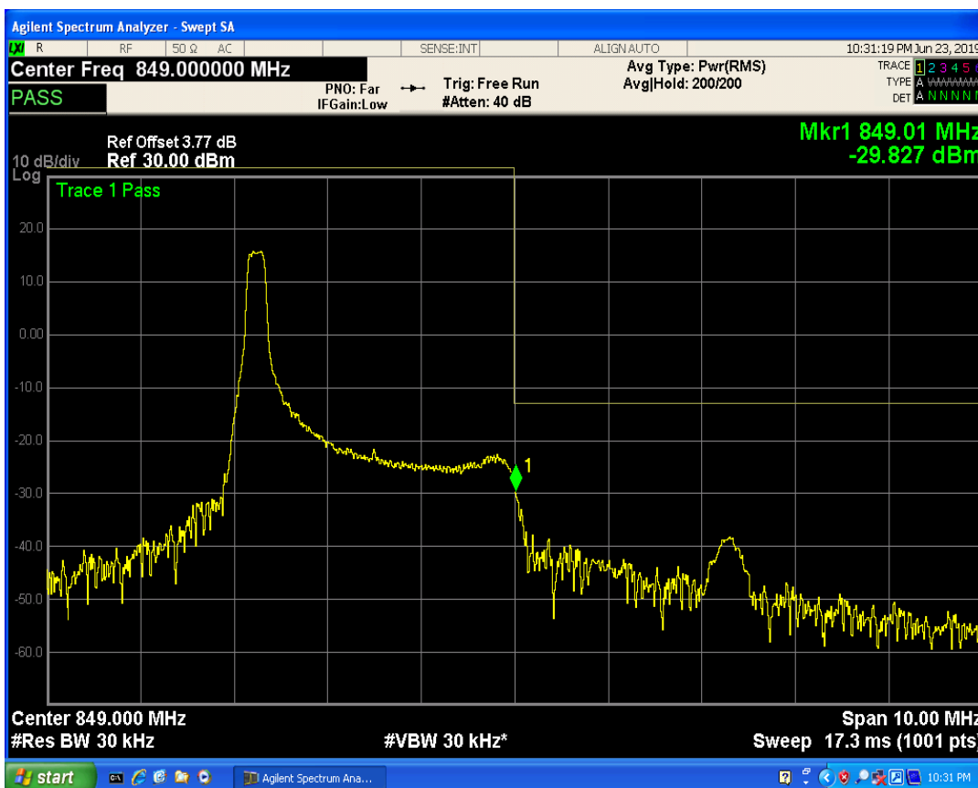
LTE Band5 QPSK BW=3MHz Channel=20635 RB Size=1 Position=#Mid
