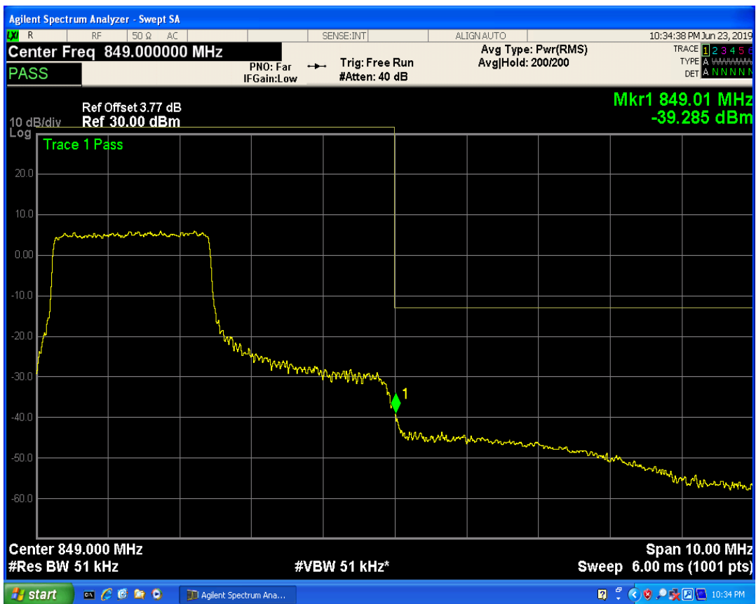
LTE Band5 QAM16 BW=5MHz Channel=20625 RB Size=1 Position=#Max
