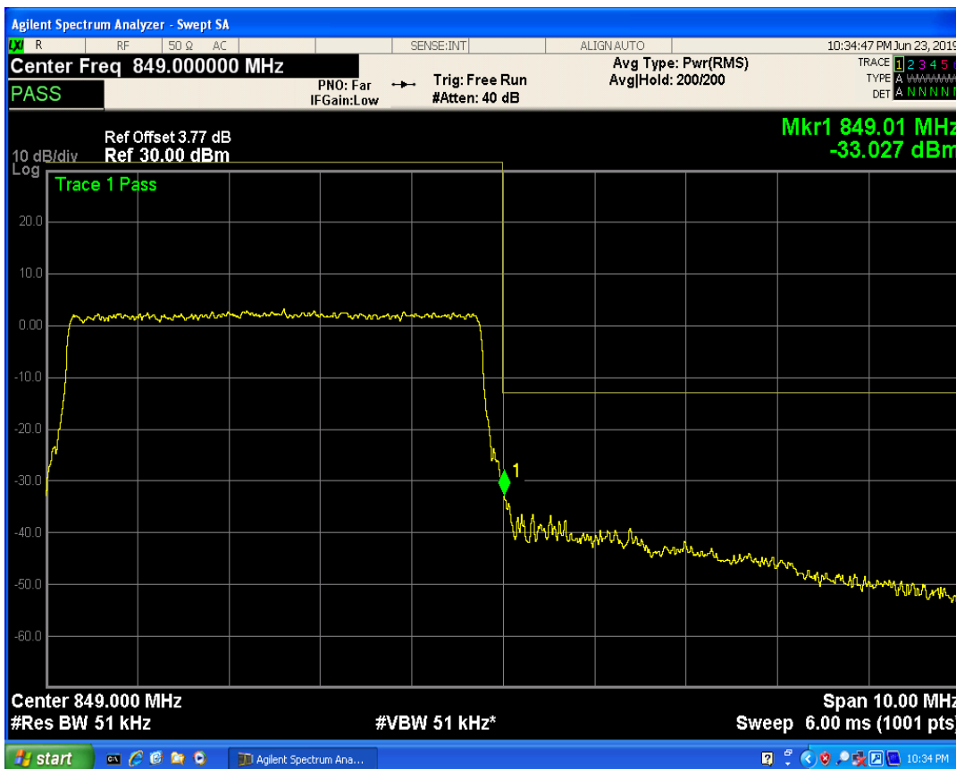
LTE Band5 QPSK BW=10MHz Channel=20450 RB Size=1 Position=#Mid
