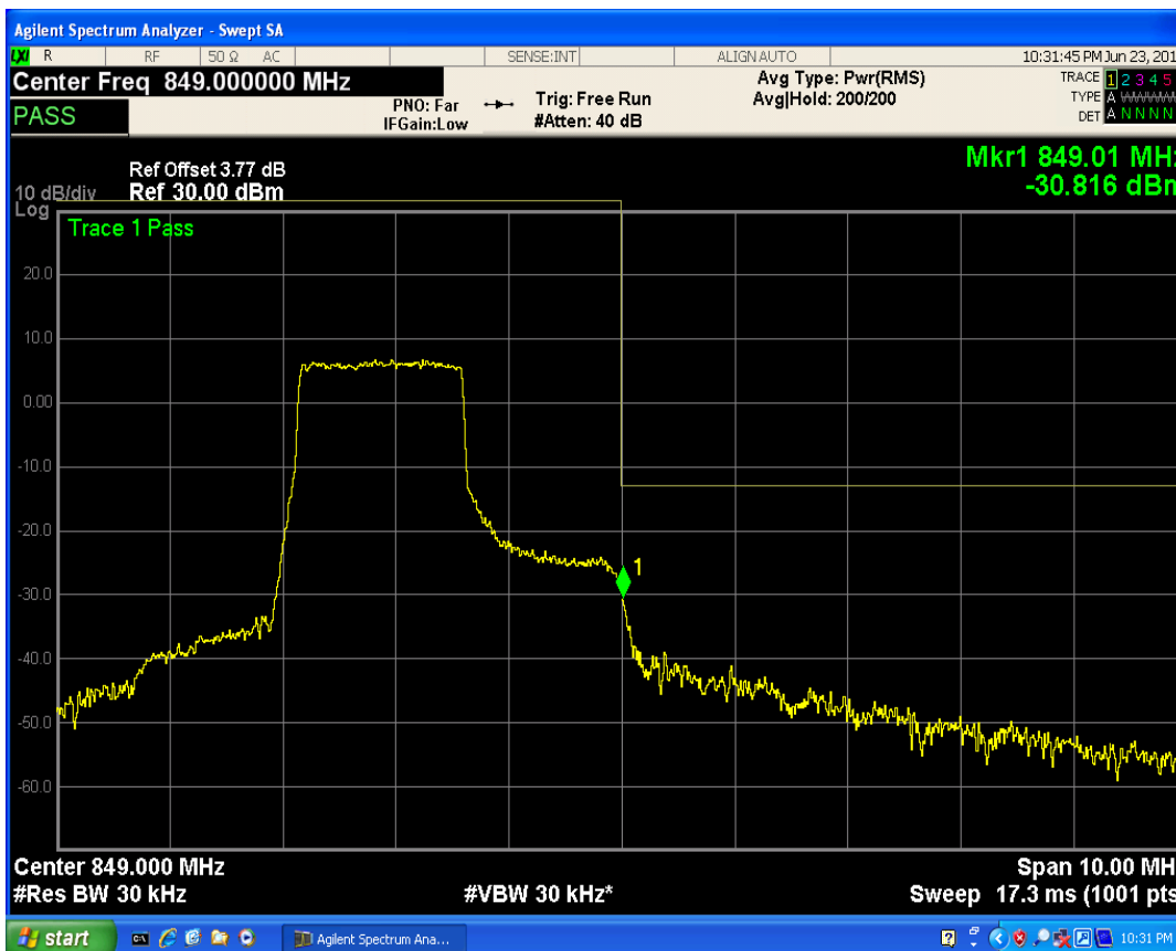
LTE Band5 QPSK BW=3MHz Channel=20635 RB Size=8 Position=#Max
