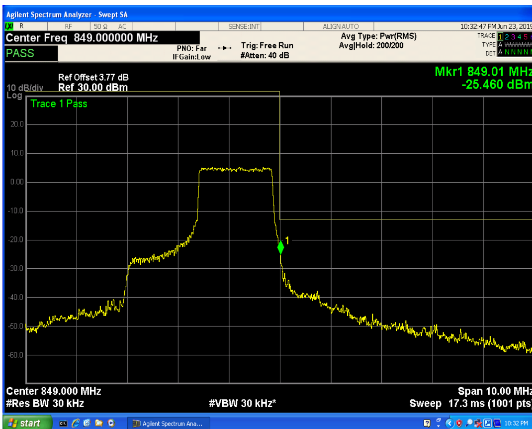
LTE Band5 QAM16 BW=3MHz Channel=20635 RB Size=15 Position=#0
