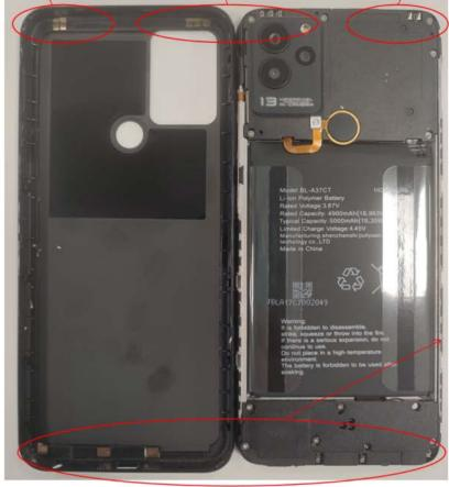
Main Antenna TX GSM B2/3/5/8; W B1/2/4/5/8; LTE B1/2/3/4/5/7/8/12/17/28/66
