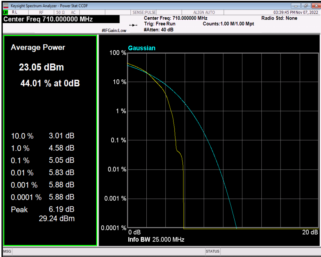
Band2 QPSK BW=1.4MHz Channel=18900 RB Size=1 Position=#0
