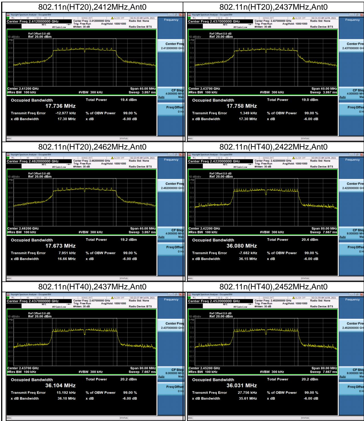
**TEST REPORT****3. Occupied Bandwidth****3.1 Test Data**
