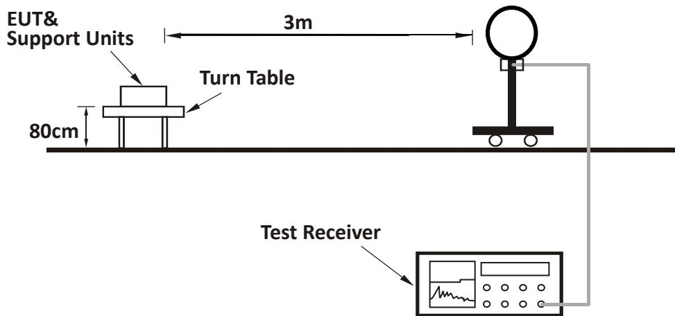
For Radiated emission 30MHz to 1GHz:
