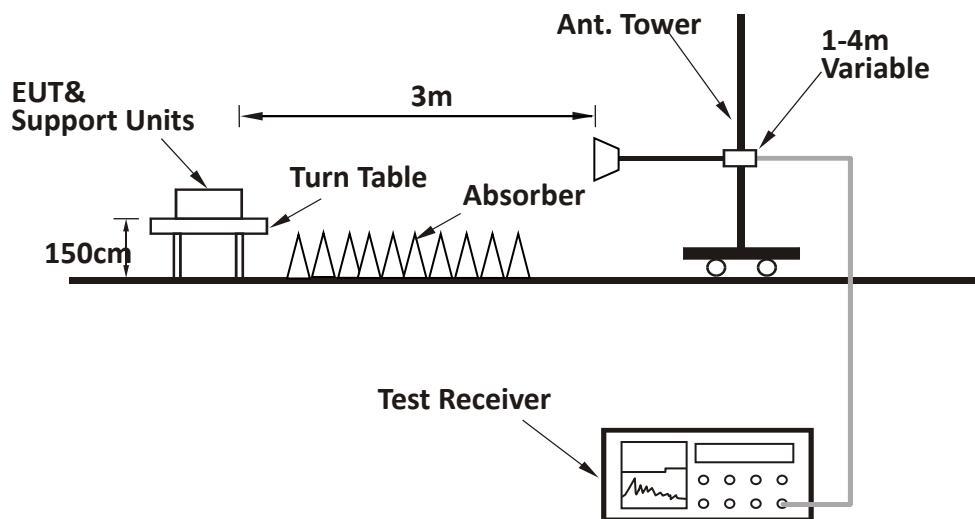
**TEST REPORT****7.4 Test Results of Radiated Emissions**
