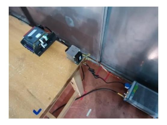
**Set-up for Radiated Emission Below 1GHz**
