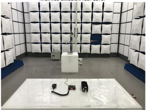
RADIATED EMISSION ABOVE 1G TEST SETUP
